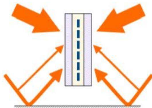
(Left) Simulated solar radiation received by a vertically mounted bifacial module and a conventionally mounted single-sided (monofacial) module during a cloudfree day in Singapore. The radiation received by the double-sided module over the whole day is more than 15% higher than the radiation received by the roof mounted single-sided module. (Right) Schematic representation of the solar illumination of a vertically installed bifacial PV module.
