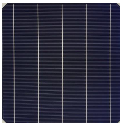
Front image of a fully screen-printed monoPoly solar cell.
