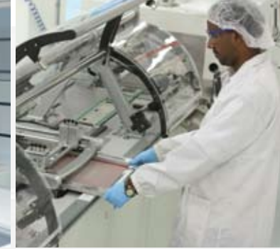
Industrial screen printer at SERIS
