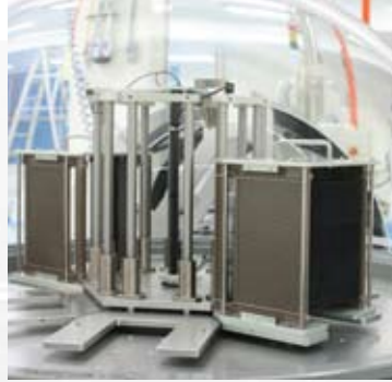
Cassette of silicon wafers at SERIS
