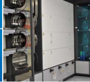
Industrial diffusion furnace at SERIS
